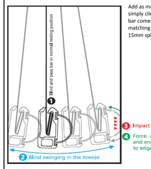
Add as many barriers as required, one for each mullion. They simply click onto the rail and can be slid to any position. The base bar comes in Clear Anodised, Black, White and Birch White with matching barriers and end caps. The Force base uses a standard 15mm spline, all available from Scottfree Australia.
