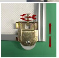
The simple turn of a screw on top of the rollers allows you to accurately align your doors with the walls every time.
